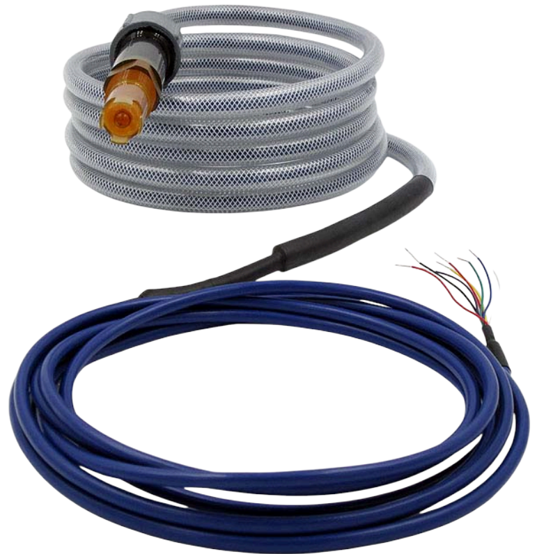
High HF-resistant submersible pH sensor with integral preamplifier (PNHF 6431) using special-order shielded and braid reinforced blue cable for use in high noise areas. Shown with a WPH seal for fully submersible use.
