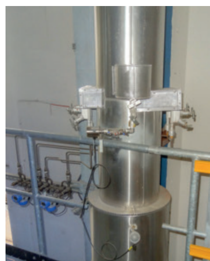
Calibrated meter run with Venturi nozzle, OPTIBAR DP 7060, OPTIBAR PM 3050 and OPTITEMP TRA-S34
