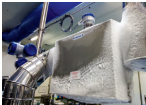
Mass flow measurement of liquid nitrogen for tunnel freezers with the OPTIMASS 6400 F
