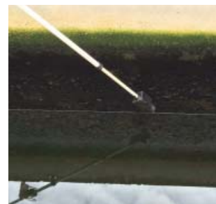
OPTISENS TUR 2000 turbidity sensor with telescopic rod holder
