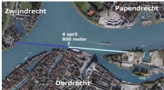
Pipeline crossing the river Merwede
