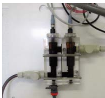
Flow cell of the OPTISYS CL 1100 with automatic cleaning
