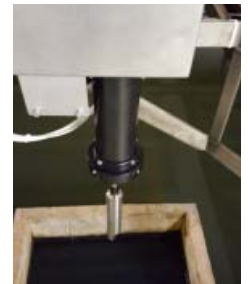
Sensor and cleaning unit of the sludge level measuring system
