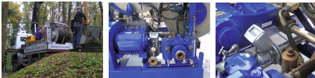
Maintenance skid with WATERFLUX 3070 for well maintenance
