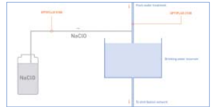
Simplified process flowsheet with measurement points of OPTIFLUX 5300 and OPTIFLUX 2100
