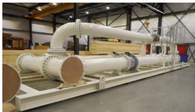
Manufacturing of water skid at KROHNE factory in Breda, the Netherlands
