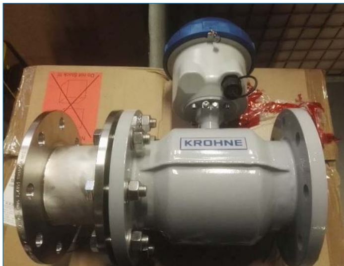
WATERFLUX 3070 with pre-fitted spool piece
