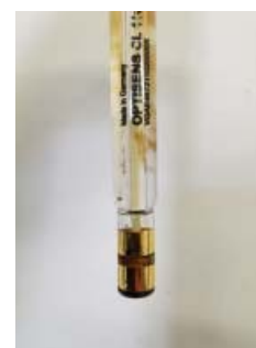
Free chlorine sensor after 8 months of operation
