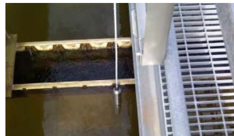
Sensor of OPTISYS SLM 2100
