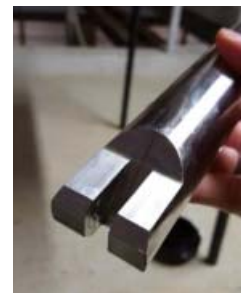
Optical sensor of the OPTISYS SLM 2100
