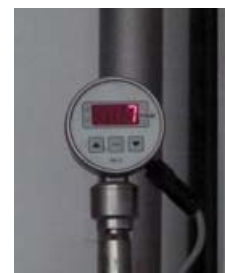
Flow measurement of methane gas at 7 mbar / 0.10 psi
