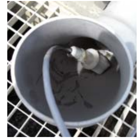
Downstream conductivity measuring device as reference
