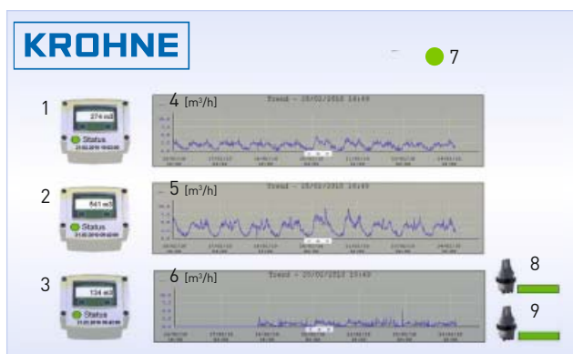
Screen shot of meter readings, current flow values and status messages
