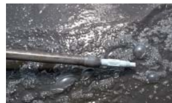
SMARTPAT ORP 1590 with integrated transmitter technology
