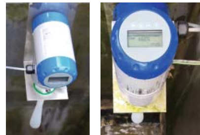
Fast retrofit of the converter thanks to quick coupling system
