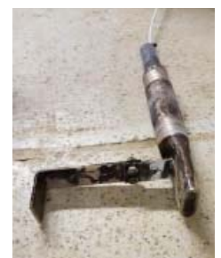
Previously used USS11 sludge level switch
