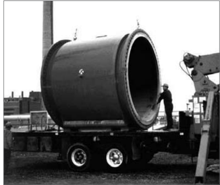
Fig. 4: World's first EMF with 3 m nominal size (KROHNE M960, 1983)
