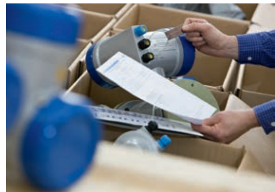
Commissioning of flowmeters
