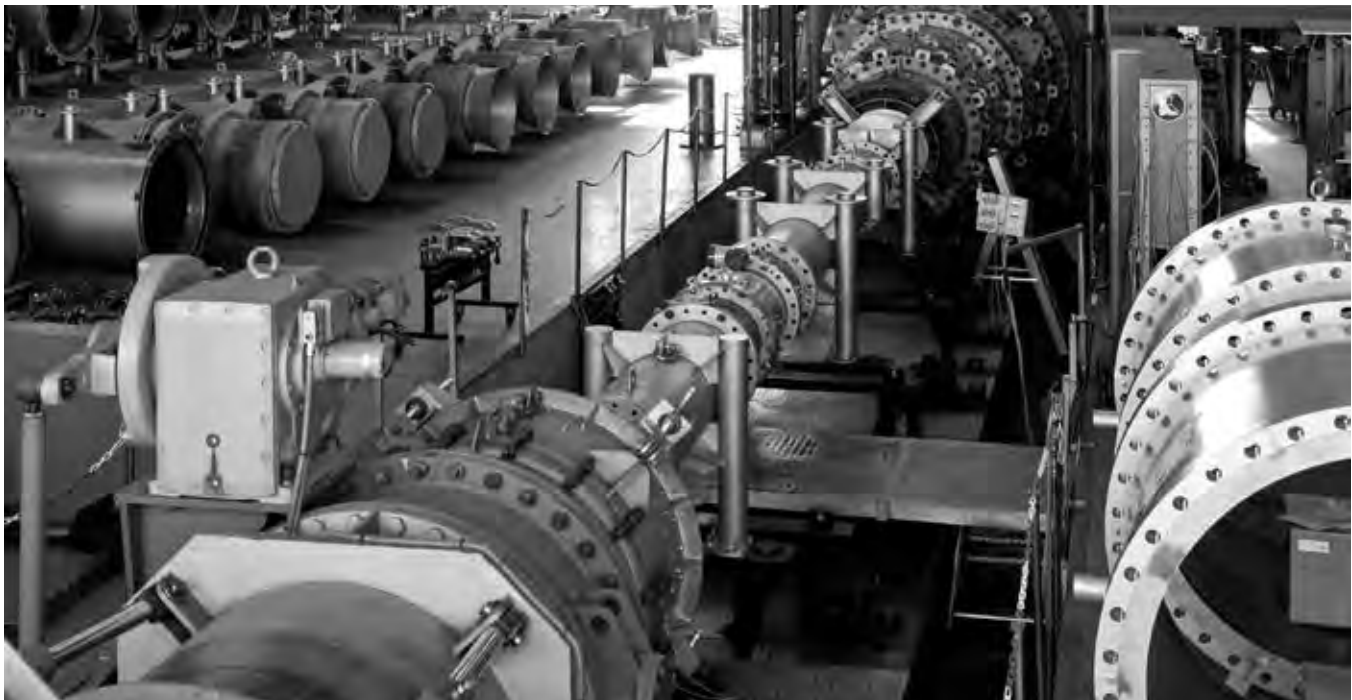
The world's most precise volumetric calibration rig for flowmeters up to DN3000/120"
