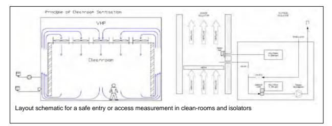
against the high concentration during the decontamination phase. The DrägerSensor HC can be used to monitor the high concentration cycle and control the start of the sampling system for the low concentration. In addition the HC sensor can show and monitor the fumigation curve.
