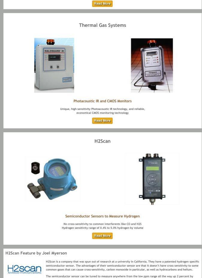
The semiconductor sensor can be tuned to measure anywhere from the low ppm range all the way up 2 percent by volume. It is a very long-life sensor - typical sensor life is ten plus years. The sensors have very little to no drift.
