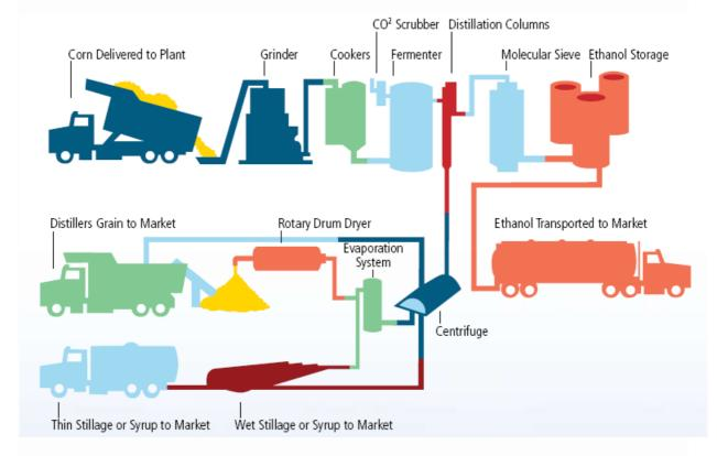
In dry milling, the entire corn kernel or other starchy grain is first ground into flour, which is referred to in the industry as "meal" and processed without separating out the various component parts of the grain. The meal is slurried with water to form a "mash." Enzymes are added to the mash to convert the starch to dextrose, a simple sugar. **Ammonia** is added for pH control and as a nutrient to the yeast.
