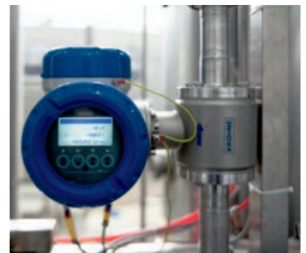
OPTIFLUX 6300 electromagnetic flowmeter
