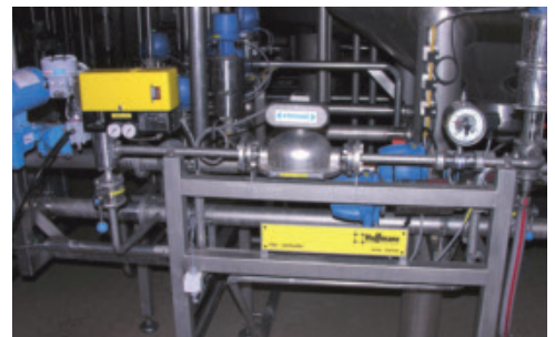
OPTIMASS 7000 F and 3000 F measuring gaseous carbon dioxide
