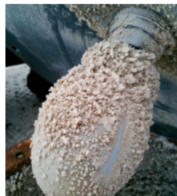
Drop antenna of the OPTIWAVE 6300: Measurement is unaffected by dust deposit
