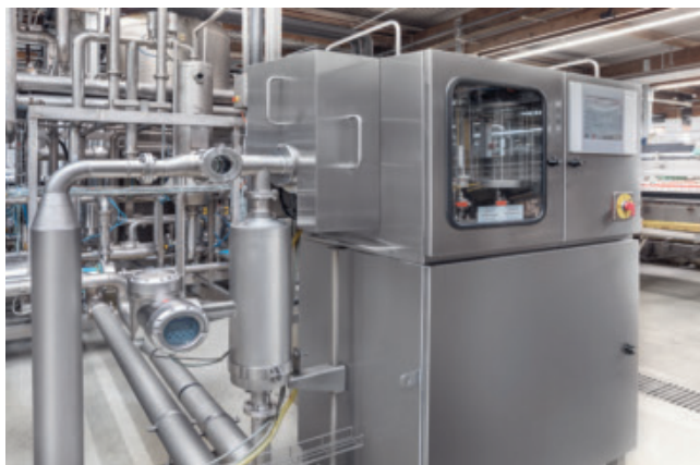
Measuring the flow of the beverage volume with the OPTIMASS 1400 C
