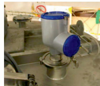
OPTIWAVE 7500 with Tri-Clamp connection
