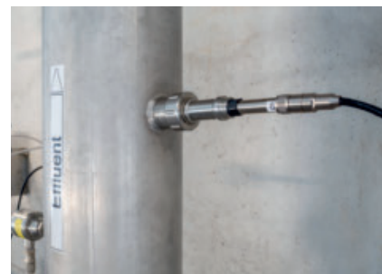
pH measurement of effluent with the SMARTPAT pH 8150
