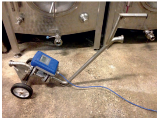
Portable measuring device incorporating the OPTIFLUX 2100
