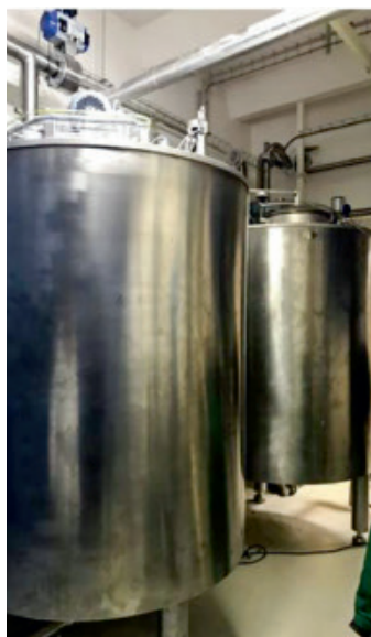
OPTIWAVE 7500 mounted on chocolate tanks
