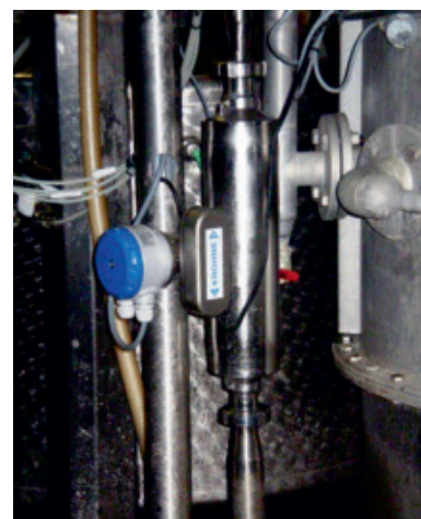
Fermented potato mash measurement with the OPTIMASS 1300
