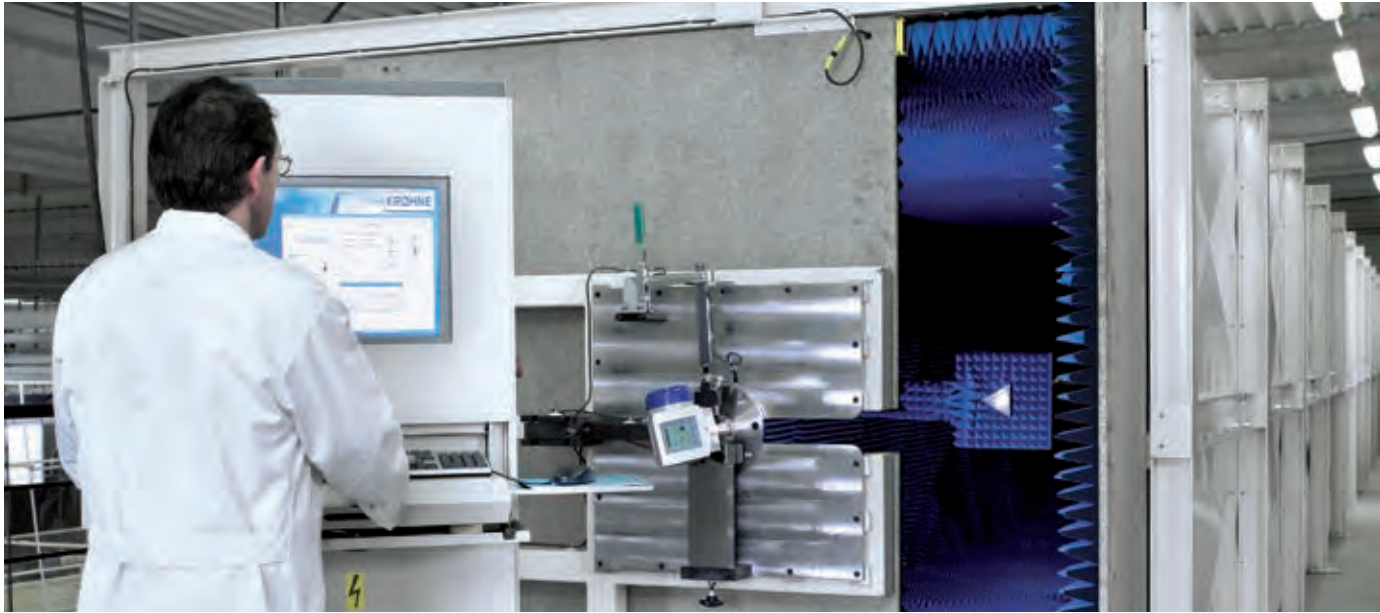
Stretch for calibration of FMCW level transmitters
