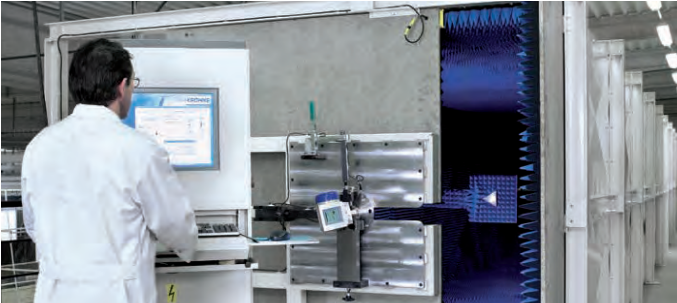
Stretch for calibration of FMCW level transmitters
