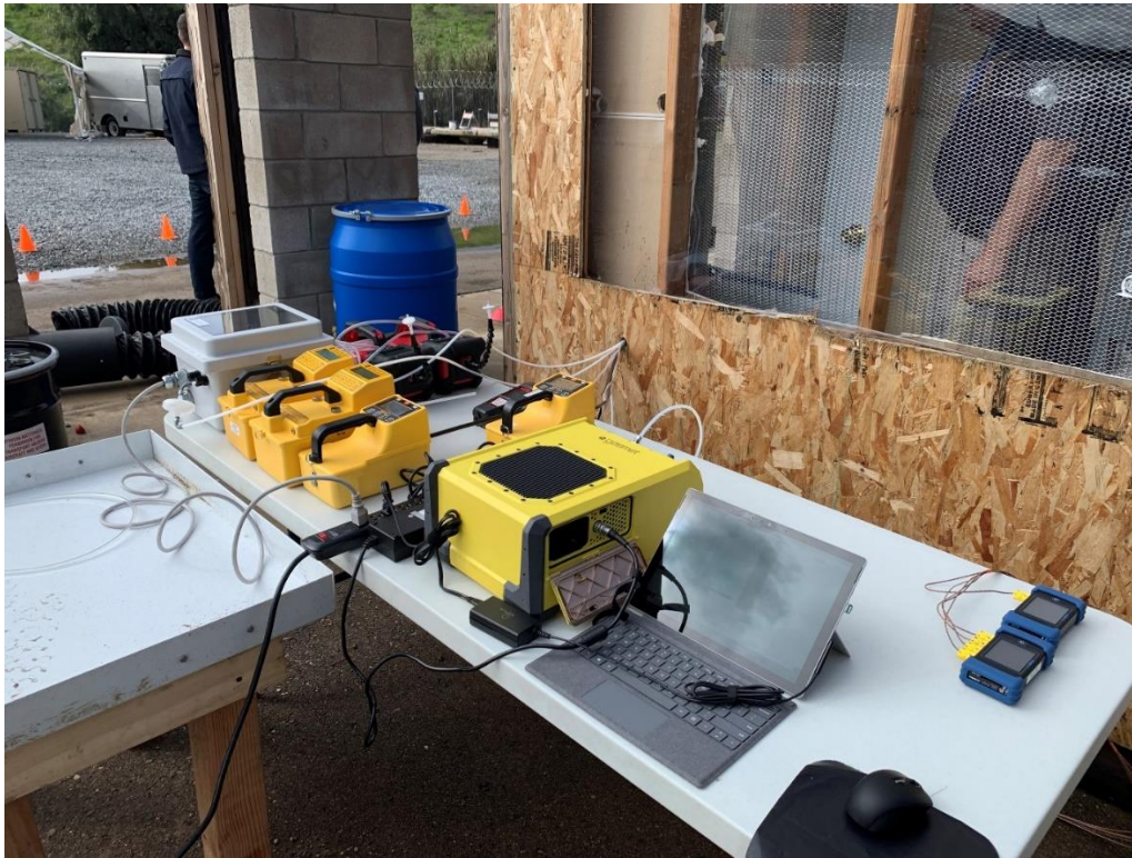
Figure 3. Gas analysis equipment employed in the research. GT5000 Terra in the center.
