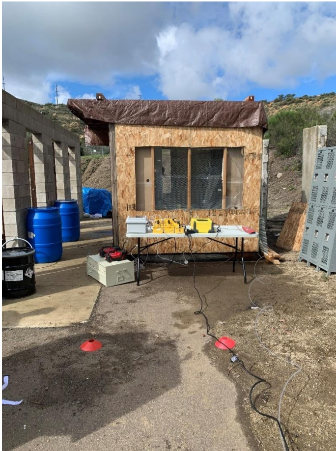
Figure 1. Wooden test enclosure. Gas analysis equipment on table in front of the enclosure.
