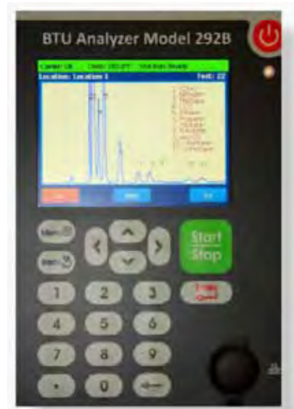
Figure 2. A Typical Natural Gas Chromatogram
