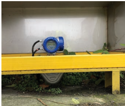
Measurement of the total hydrogen consumption with the OPTIMASS 6400 Coriolis mass flowmeter (DN15)
