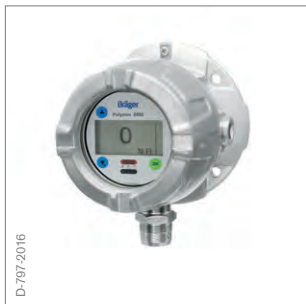
Dräger Polytron® 8200 CAT Explosion-proof transmitter with optional relays and bus communication uses a high performance catalytic bead DQ sensor
